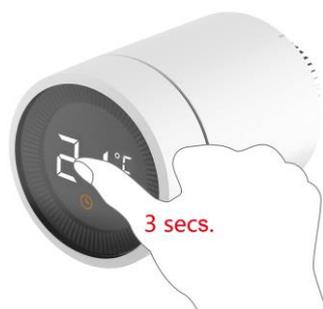
1) Press the knob and hold on for 3 seconds before the product be installed on the valve.
